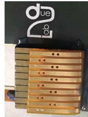
Fig. 1. Overview of the cathode electrode bonding of the 3D drift strip CZT detectors.
